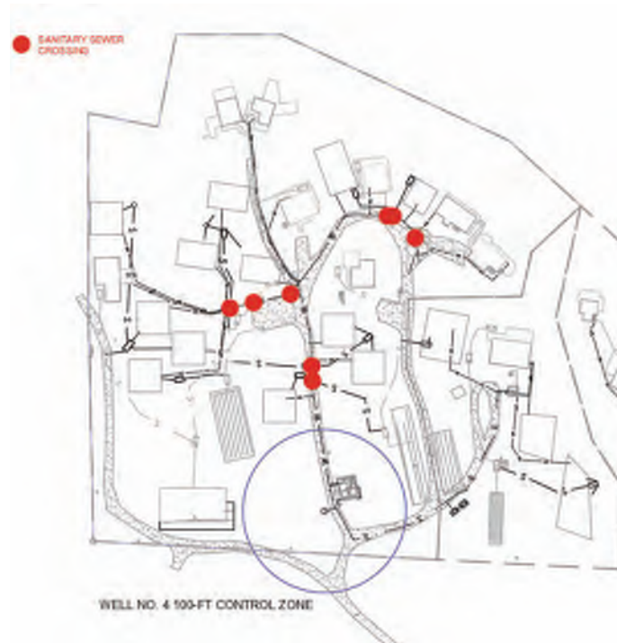
FIGURE 2. PWS SANITARY SEWER CROSSINGS
